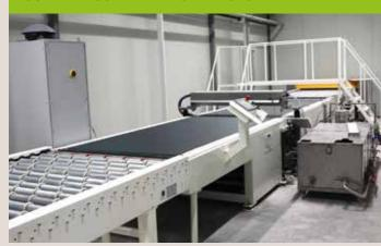
**CURTAIN COATER MACHINE SYSTEM,** Wouldn't you like to apply curtaining without any material loss at a speed of up to 15 meters per minute and with minimum labor?
